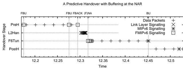
Fig. 4. Packet loss and handover latency for a predictive handover
