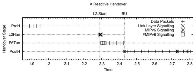
Fig. 6. Packet loss and handover latency during a reactive handover.
