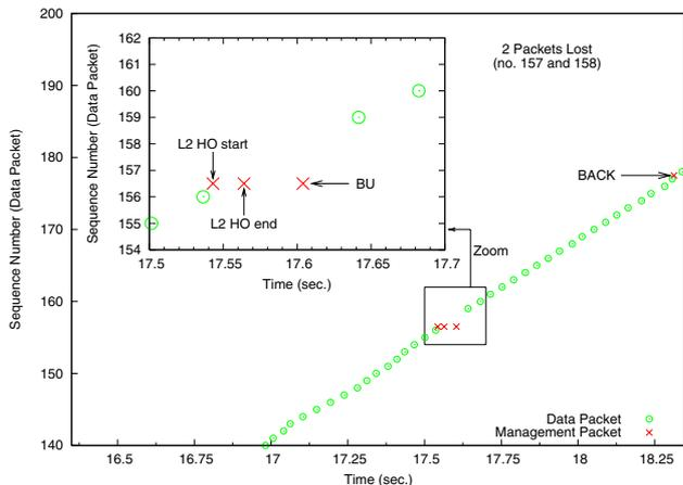
Fig. 3. Impact of the MIPv6 protocol on a Video Stream
