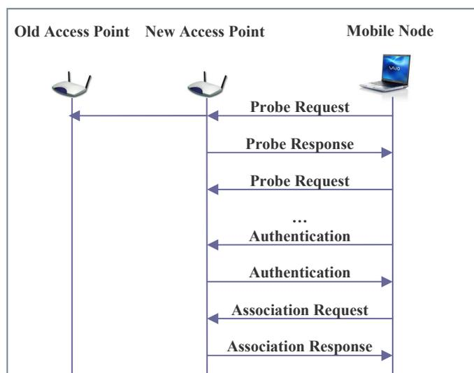
Figure 1. The WLAN Association Process (Active Scanning)
