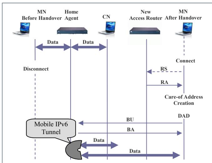
Figure 2. Mobile IPv6 Operation and data forwarding
