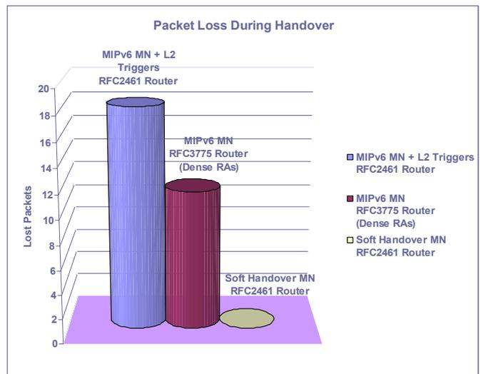
Figure 7. Packet loss during handover.
